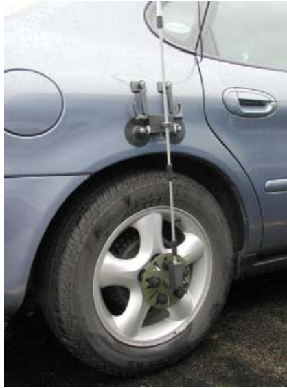
Holding Plate with Suction Cups and Magnets
