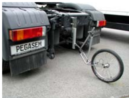
Flange Adapter fixed to under-floor bars
