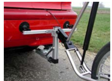
Firm and secure attachment using the towing lug
